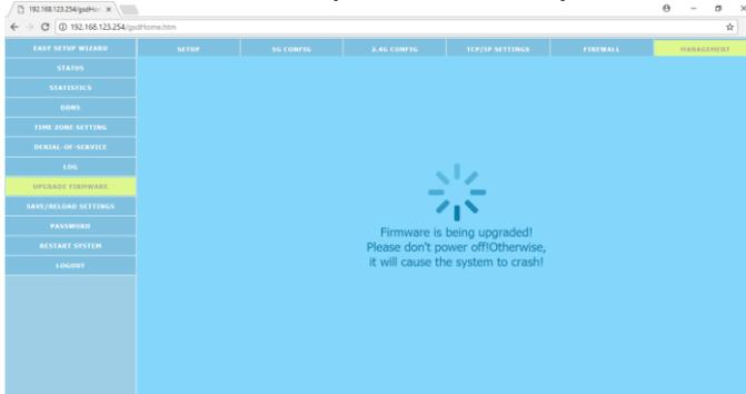
During the upgrade, the router is rebooting automatically. That means that Leddura 2Meet is reporting Network disconnected and connected several times. This is perfectly normal and as expected. Just wait until the upgrade is done. Upgrade time can take 5~10 minutes so please be patient.
