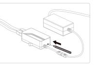
If you notice that the remote does not pair, press the small button on the side of the control box with a paper clip or pencil as shown. Once the lift stops beeping, press the "SET" button on the remote control. You should hear consecutive beeps for around 10 seconds indicating the pairing is ongoing. After that the lift beeps once more, indicating that the pairing is completed. Now calibrate the lift as written above.
