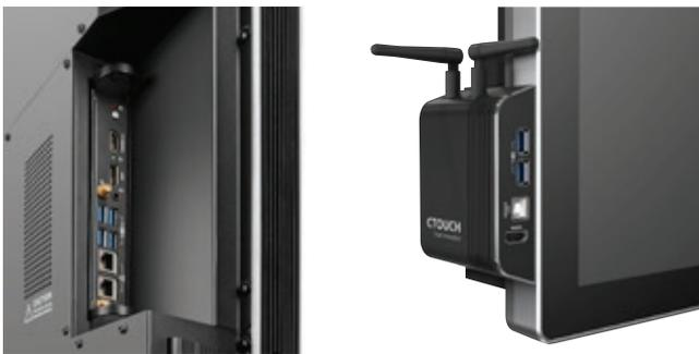
The OPS module is an Intel® OPS compliant mini PC for Interactive Touch Displays and Digital Signage applications.
