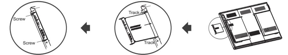
2. Fasten the internal PC module with two screws provided on the side frame of the CTOUCH interactive display.
