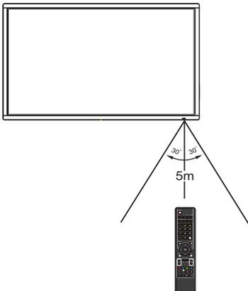
Use the remote control by pointing it towards the remote sensor on the front of your CTOUCH interactive display. Objects between the remote control and the remote sensor may prevent proper operation.
