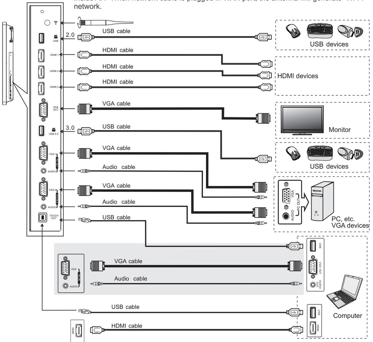
Connect PC with VGA cable or HDMI cable.
