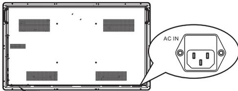
1. Connect the female plug to the AC socket on the unit.
