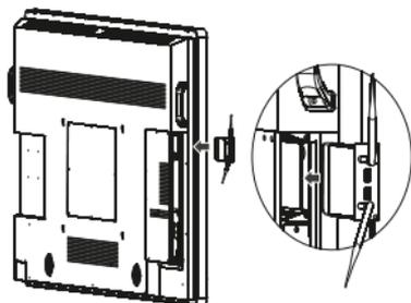
2. Tighten the Wi-Fi antennas in clockwise direction and insert the Wi-Fi module in the Wi-Fi slot.
