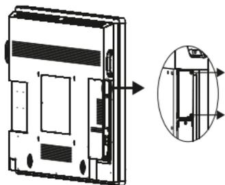
1. Remove the screws and take the plate out. Keep the screws in a safe location, as you will need them later on.
