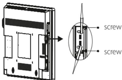
3. Fasten the Wi-Fi module by turning the screws back in place.
