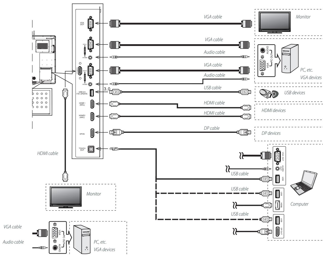
Connect TOUCH OUT with USB cable to PC USB port.
